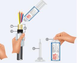
Re-insert the barrier pot sub-assembly 5 back into the nipple nut 2.
