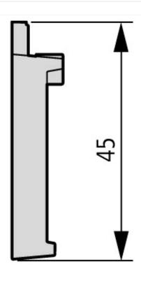
mounting clamp Fixing adapter (front mount) for 4
