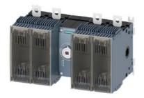
Switch disconnector with fuse 250 A, Size 3, 4-pole for LV HRC fuse Sz. 0 and 1 Front operating mechanism center Basic unit without handle flat terminal
