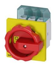
SENTRON, Switch disconnector 3LD, emergency switching-off switch, 3-pole, lu: 32 A, operating power / at AC-23 A 400 V: 11.5 kW, front-mounted, rotary operating mechanism, Red / yellow, 4-hole mounting of the handle
