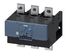
Overload relay 160...630 A for motor protection Size S10/S12, Class 10E Contactor mounting/stand-alone installation Main circuit: busbar connection Auxiliary circuit: Spring-type terminal Manual-Automatic-Reset
