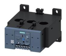
Overload relay 50...200 A for motor protection Size S6, CLASS 5...30E Contactor mounting/stand-alone installation Main circuit: straight-through transformer Auxiliary circuit: Screw terminal Manual-Automatic-Reset Internal ground fault detection
