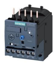
Overload relay 1...4 A Electronic For motor protection Size S00, Class 10E Contactor mounting Main circuit: Screw Auxiliary circuit: Screw Manual-Automatic-Reset
