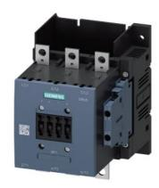
Power contactor, AC-3 185 A, 90 kW / 400 V without coil Auxiliary contacts 2 NO + 2 NC 3-pole, Size S6 Busbar connections Drive: conventional Auxiliary conductor: Screw terminals
