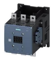
Power contactor, AC-3 400 A, 200 kW / 400 V without coil Auxiliary contacts 2 NO + 2 NC 3-pole, Size S12 Main conductor: Busbar connections Drive: conventional Auxiliary conductor: Screw terminals
