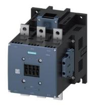
power contactor, AC-3 500 A, 250 kW / 400 V AC (50-60 Hz) / DC 110-127 V AC/DC auxiliary contacts 2 NO + 2 NC 3-pole, frame size S12 busbar connections drive: conventional screw terminal
