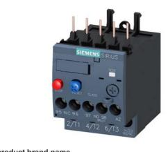
Overload relay 0.70...1.0 A Thermal For motor protection Size S00, Class 10 Contactor mounting Main circuit: Screw Auxiliary circuit: Screw Manual-Automatic-Reset
