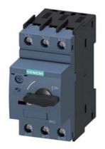
Circuit breaker size S00 for transformer protection A-release 2.8...4 A N-release 82 A screw terminal Standard switching capacity
