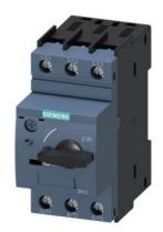
Circuit breaker size S0 for transformer protection A-release 13...20 A N-release 325 A Screw terminal Standard switching capacity
